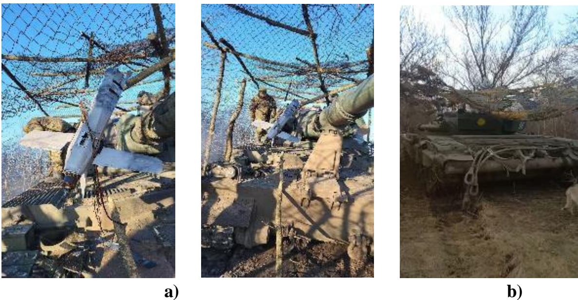
Figure 3.6 – An example of the use of metal nets as protective screens by artillery units (a) and tank units (b)
