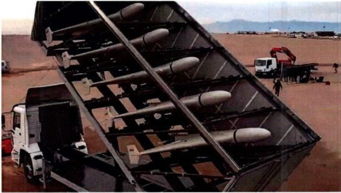
Figure 1.3 – Puskova installation UAV "Shahed 136", disguised as a dump truck
