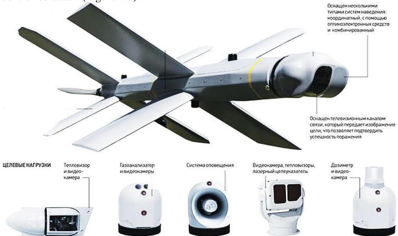
Figure 1.5 – Equipped with several types of guidance systems and a combined television communication channel
