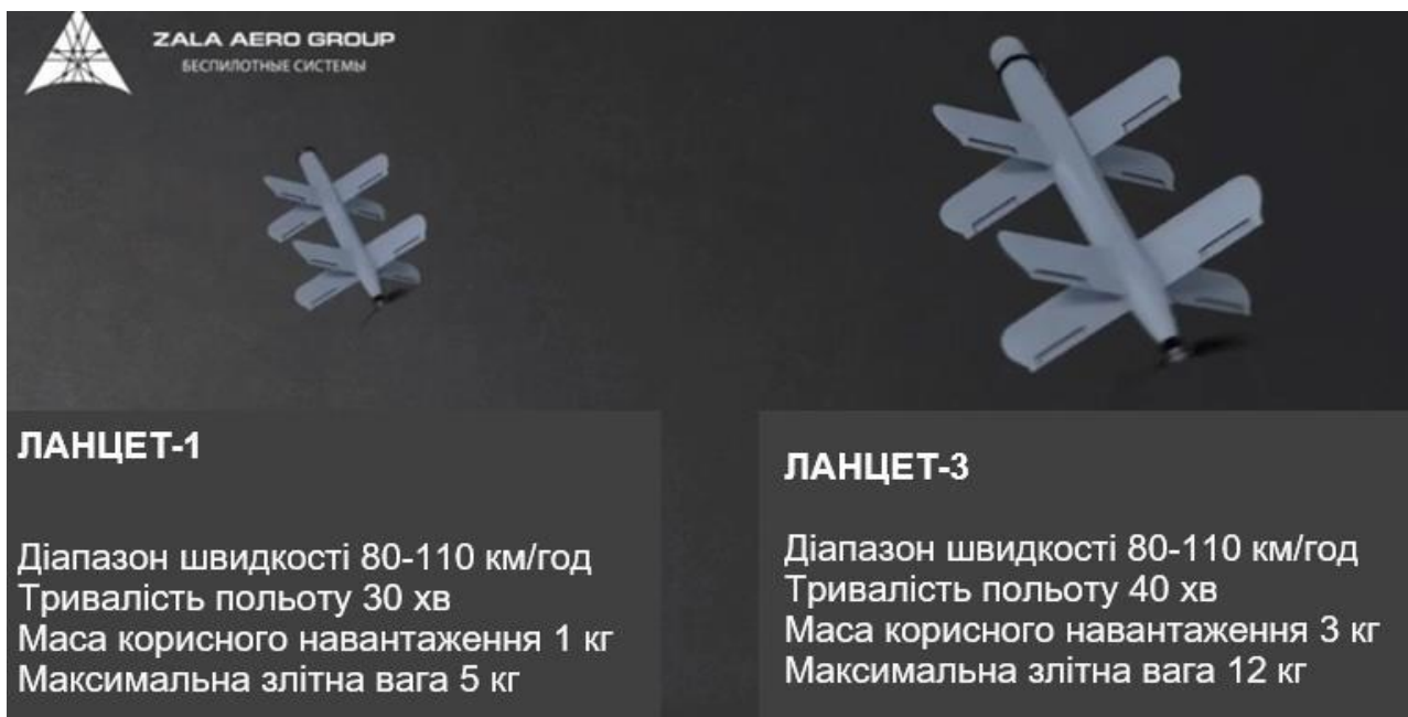
Figure 1.4 – Characteristics of shock UAVs "Lancet - 1" and "Lancet - 3"
